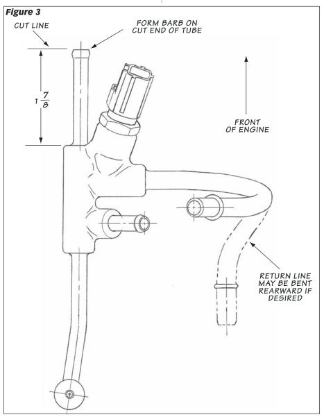
the sensor removed, Deburr cut end of tube on the cluster, rinse assembly with solvent and blow dry. Reinstall sensor
