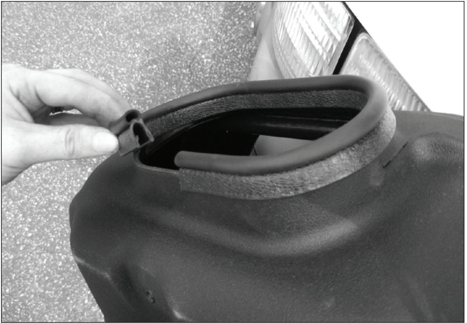
Figure 5- Attachment of Edge Grip Seal
