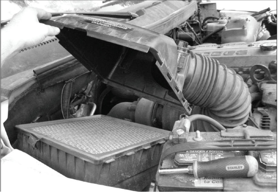
Figure 4- Removal of filter housing bottom
