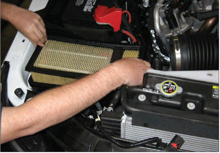
Figure 5-Removing stock air filter element
