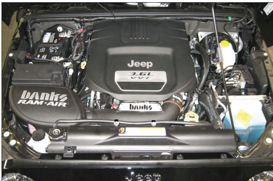
Figure 8- Installed Banks Ram-Air Intake System
