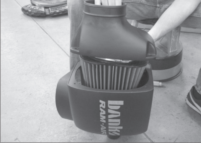
Figure 10- Inserting Banks Air Filter Cover into Banks Air Filter Housing
