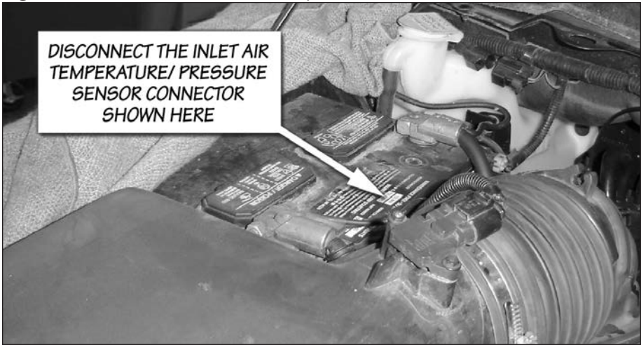
Figure 1. Location of the Inlet Air Temp/ Pressure Sensor
