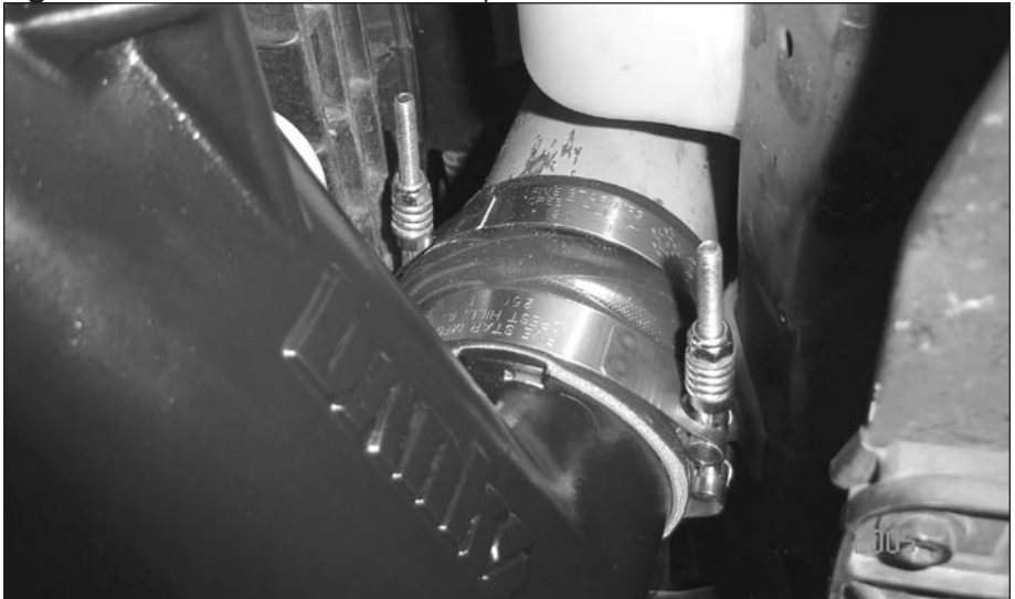
Figure 7. Orientation of the Hose Clamps on the Driver Side.
