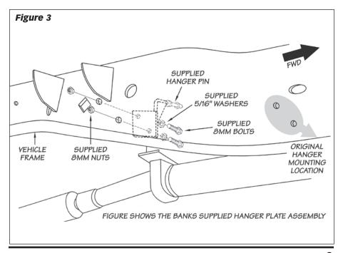
A) Using a pry bar, completely remove the rubber hanger from the front muffler hanger pin. Remove the two (2) factory nuts on the front muffler hanger pin from the frame rail and remove the hanger pin from the vehicle. Retain the rubber hanger for re-assembly.
