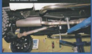
4 Matthews installed the 4-inch pipe by connecting it to the catalytic converter, where the new exhaust system starts.
