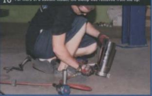
12 With the clamp removed, the tip was welded on for a clean installation.
