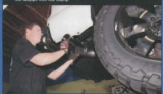
11 Matthews cut off approximately 3 inches of the tailpipe so the tip would not protrude from the truck as much as the clamped install. The shorter tailpipe gives the truck a cleaner look while still allowing the striking polished tip to be seen.
