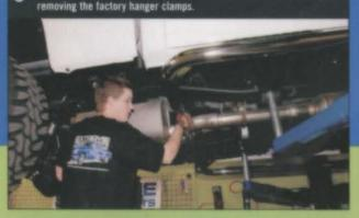
5 The new, wider, polished stainless steel muffler was attached to the intermediate pipe to dissipate the midrange exhaust drone. It features a straight-through, 4-inch-diameter flow path with a Banks-designed expansion chamber.
