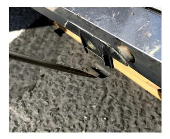
3. Now that the top two fasteners of each OEM fog light assembly are exposed, the bottom bolt on each will need to be addressed. These bolts can be found underneath the vehicle on the backside of the front bumper. There is a small rubber flap that can be pushed away to access the bolts. If needed, use a standard screwdriver to pry up the plastic fasteners holding the flap to the bumper. Below is an image of the OEM fog light bracket for reference.
