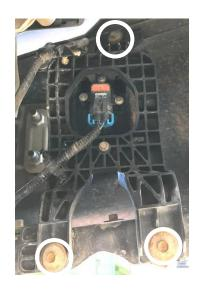
3. Locate the stainless-steel Super Duty brackets and the Squadron parts bags. With the 4mm Allen wrench, screw in the Squadron 6mm housing bolts through the washer, bracket, serrated washer, and then into the light housing. Repeat step for the opposite side of the housing, then repeat for the other light. The exploded view below is for reference.
