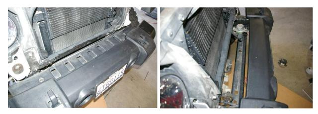
Note: The black plastic piece can be a little tough, but once you have removed the fasteners you can twist the plastic piece and pull it out to the side.
