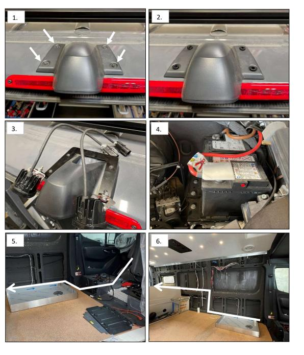
7. Once the rear doors are reached, route the wires through the OEM door wiring pass through. Use silicone or any sealant to prevent leaks in the rubber. Route the wires up the door seal to the lights, Use the supplied splitter harness to attach the two lights to the harness.
