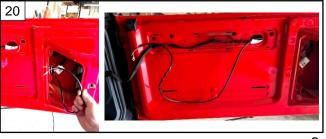
21. Zip tie the license plate harness to the OEM swing gate harness as shown. Replace both the the swing gate panels from step 15.
