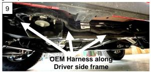
10. The main harness (upfitter or toggle switch) will need to be unraveled. Route the light lead of the harness down the driver side firewall away from any hot, sharp, and/or rotating components. Continue routing the harness until it reaches the 10ft extension. Connect the main harness lead to the extension. Remove the slack and tie the harness as needed, pulling up into the engine compartment. Any extra harness length can be tied up and placed into the inner driver side fender.
