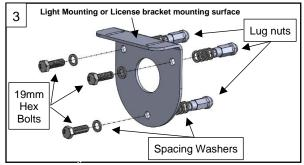
adjustment for different wheel styles/offsets. The included 19mm hex bolts are M12 x 1.5 x 40mm. Mockup the reverse bracket with the top flange facing away from the spare tire. Determine the correct number of washers needed in-between the bracket and lug nuts are needed to clear the wheels. Tighten the bolts.
