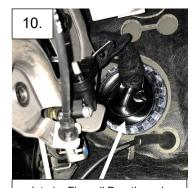
Interior Firewall Passthrough (Use lube when reinstalling)
