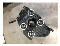
4. Using the 3mm Allen wrench, remove the four Bezel bolts (circled below) that hold on the standard Squadron bezel. Replace the bezel with the provided Super Duty bezel and retighten hardware. With the 4mm Allen wrench, screw in the Squadron housing bolts through the washer, bracket, serrated washer, and then into the light housing. Repeat for the opposite side of the housing.
