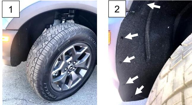
2. With the trim tool, or flathead screwdriver, remove the five plastic fasteners in the front of the driver side wheel well. With the 7mm socket, remove the single fastener on the underside of the bumper.
