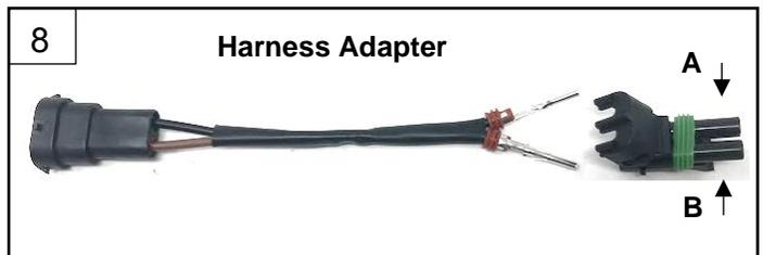
9. Turn vehicle off. Plug in the wiring adapter. Trace the (+) wire through the harness adapter. The (+) wire will need to be inserted into the provided plug in the (B) pin location. The ground will then be inserted into the (A) location.
