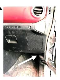
Tie wires away from all sharp, hot, and/or rotating components.
