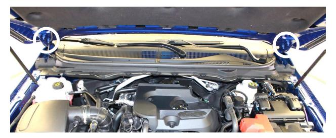
2. Place masking tape along the hood hinges (shown below) to ensure proper realignment. Also, place masking tape along the back edge of the hood near the windshield to prevent any scratches when aligning the bracket.
