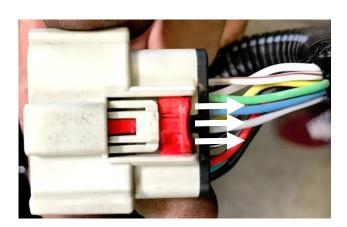
7. To disconnect the taillight plug, pull the red tab up until it appears as the picture on the right above. Now press the white detent in and pull the plug from the light.
