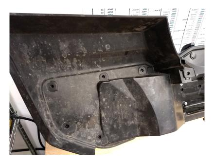
Step 2: Unplug factory fog lights and remove the three screws holding lights to bumper.
