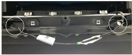
4. With a Standard screwdriver (flathead), bend all the bumper cover mounting clips back to original condiditon. Before picture on left below, after on right.
