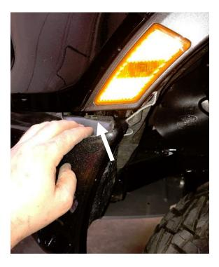
4. Unplug the OEM fog lights. Locate the four T25 head Torx bit fasteners that mount the light assemblies (Pictured below). After removing the screws, remove the lights.
