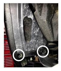
2. Fold back the rubber flap inbetween the front bumper and fender shown below. Carefully pull back the upper inner fender well to reveal the top of the fog light back splash. Repeat for passenger side.
