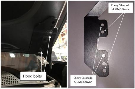
Note: Do the driver and passenger side independently so the hood does not become misaligned.
