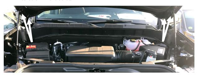
2. Place masking tape along the hood hinges (shown below) to ensure proper alignment.
