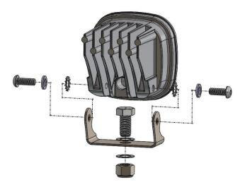
10. Now with the 9/16" wrench and socket, the lights can be placed onto the A-pillar brackets, aimed, and tightened.
