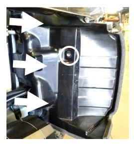
9. Locate the three bolts on the driver side Aluminum front bumper structure. The two circled in the picture below will be used to mount the bracket. With a 14mm socket wrench, remove the bolt closest to the center of the vehicle, then loosen the bolt right next to it until it is about ¼" above the surface of the black plate.
