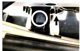
12. Locate the brackets and rubber pads included with the kit. Remove adhesive film and place the pads on the bottom foot of each bracket. See the "PS" (Passenger Side) bracket below for reference. Trim any excess rubber.
