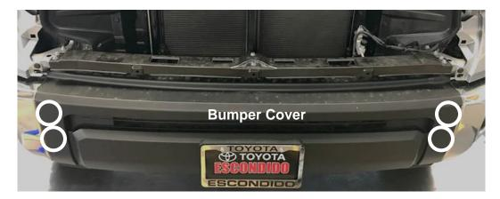
10. With the Flathead screwdriver, pry up the plastic fastener on the center of the bumper cover and remove. Now the bumper can be lifted and removed. Place the cover on a soft surface.
