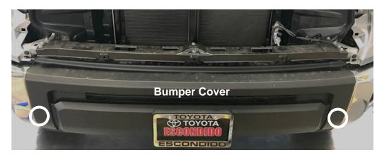
Carefully pull down the bottom edge of the bumper cover so you can access behind the circled fasteners shown above. With the 10mm wrench, reach into the back of the bumper near the bottom left or right and carefully loosen the nut. It should easily come off by hand after breaking loose with the wrench. Repeat for the opposite side. (Passenger side nut arrowed in image next to step 7)
