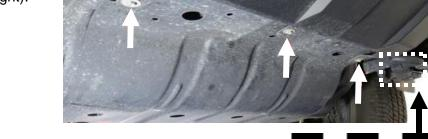
7. With the 10mm socket wrench, remove the two nuts on the bottom corners of the bumper cover (one per corner). Carefully push the bumper forward enough to free the stud (See passenger side image on right with fastener circled).
