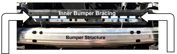
Mask off the bottom edge of the inner bumper bracing. Carefully reach behind the bumper cover in between inner bumper bracing and bumper structure to reach the four fasteners with the 10mm socket wrench (circled below). Reposition if needed. Break the nuts loose and finish the removal by hand.
