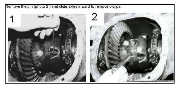
Remove the axles, taking care not to damage the seals. This is a good time to inspect the seals, axles and bearings, replacing as necessary. Also, measure the outside diameter of the axle flange. To properly seat in the rotor, the flange diameter can not exceed 5.9". If yours is larger, a machine shop can turn these down for proper fit.
