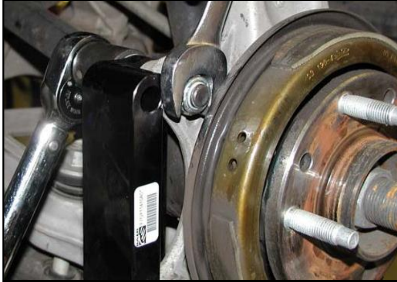
Figure 2: Installation of the intermediate bracket
