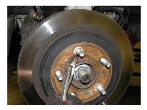
Thoroughly clean the hub and caliper mounting surfaces to assure the new Baer components will seat properly.
