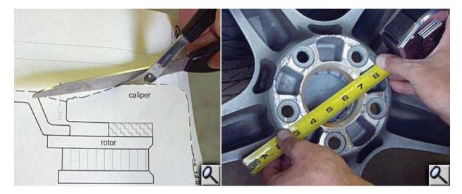
After you have cut the template along the bold dotted line, measure the inside diameter of the wheel where the hub goes inside the wheel. The wheel in this photo has a chamfer at the top of the hub hole.
