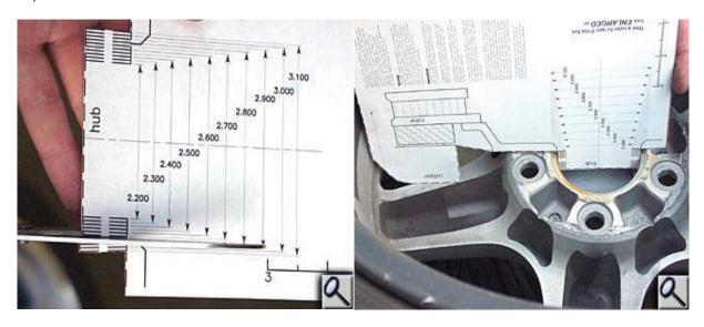
Once you have trimmed the hub area of the template, place the template into the back of the wheel. The hub area of the template should fit down into the hub hole in the wheel. This "Extreme" system template fits into this wheel with one exception; the template is resting on the spoke of the wheel and not allowing the template to rest flat on the hub section of the wheel. Also note that the template is very close to hitting at the top of the wheel to the top of the caliper.
