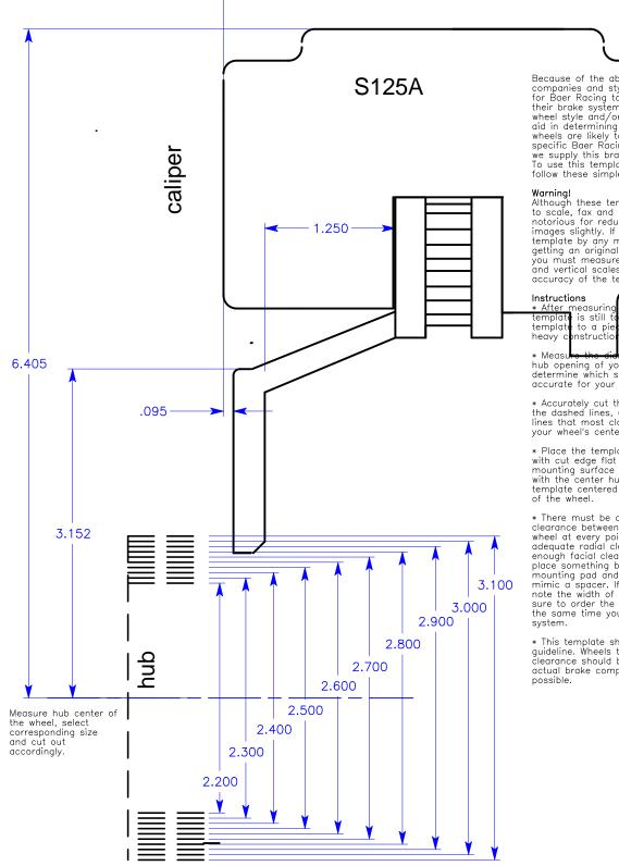
Because of the abundance of wheel companies and styles, it is impossible for Baer Racing to guarantee ft of their brake systems into a specific wheel style and/or manufacturer. To aid in determining for yourself f your wheels are likely to fit around a specific Baer Racing brake upgrade, we supply this brake system template. To use this template to determine fit, follow these simple instructions
