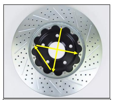
4. Using an in lb torque wrench and a hex socket, torque each Fastener to 180-200 in lbs. or 15-16 ft. lbs. Use an alternating star pattern when torqueing rather than in a continuous series around the perimeter of the Rotor.
