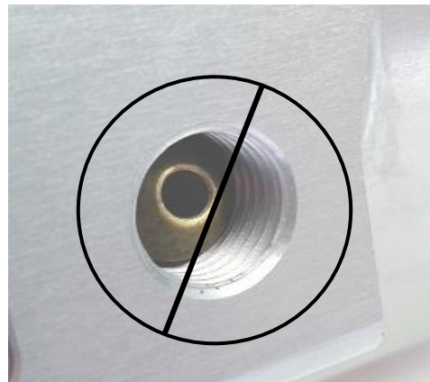
Figure 5: Insert incorrectly installed
