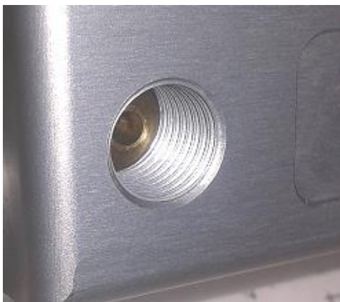
Figure 4: Insert correctly installed
