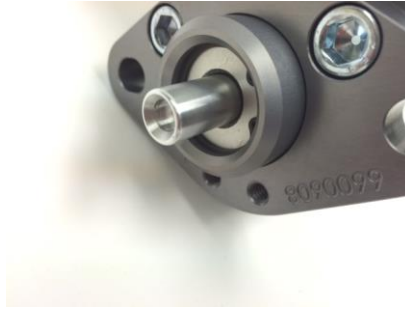
Figure 2: Master cylinder bullet (short pushrod booster)
