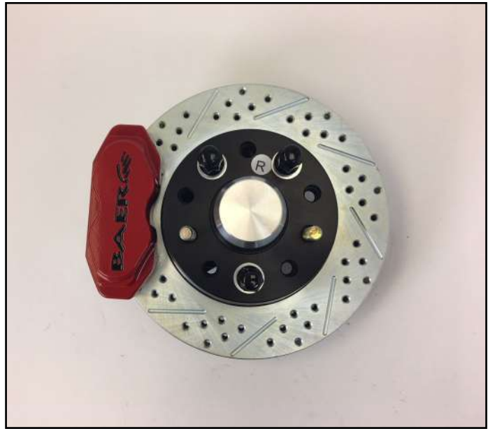
8. Outboard view of caliper installed. Now refer to the shimming portion of these instructions.
