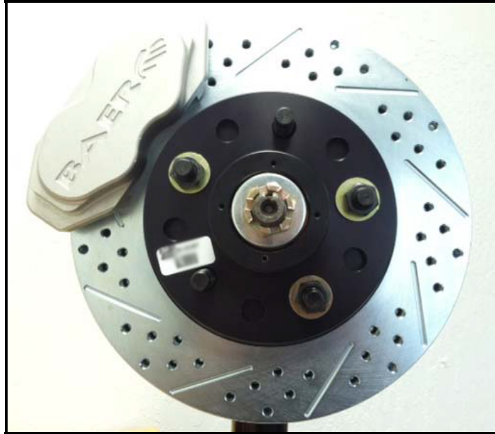
Figure 5: Caliper and rotor installed
