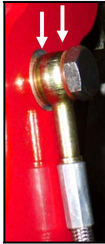
Figure 8: Installation of brake hose and washers
