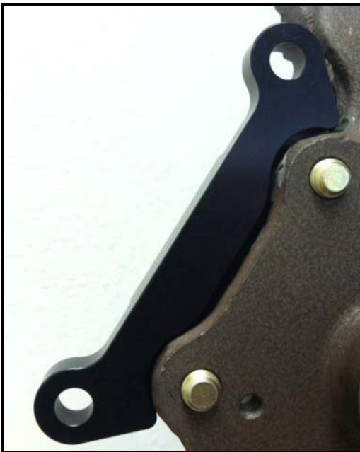
Figure 3: Bracket installed onto passenger side (right) spindle
