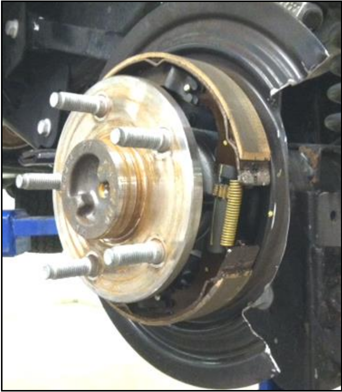
Figure 3: ¾ view of the dust shield trimmed for caliper clearance
