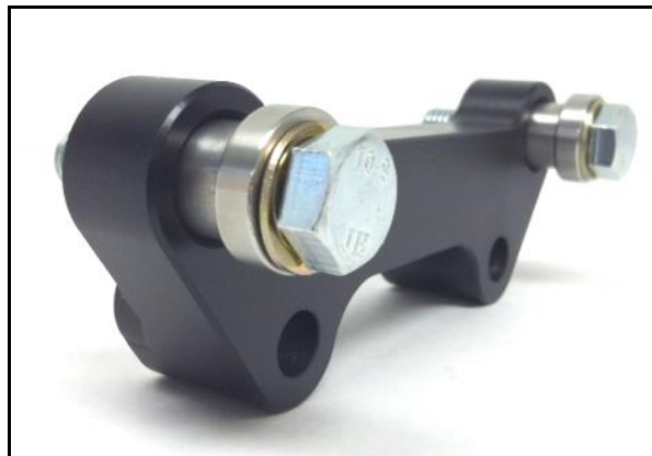
Figure 6: Correct installation of bolts, washers, and slider pins
