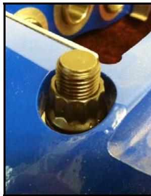
Figure 10: ARP studs, washers, and nuts installed
