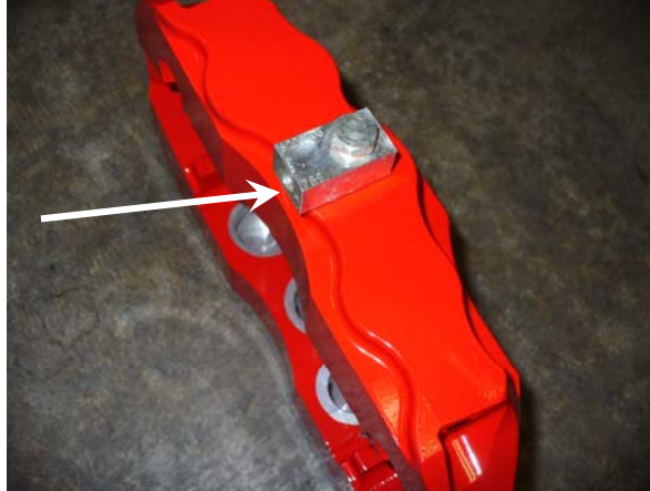
Adaptor attached to caliper. Fluid opening faces inboard.
