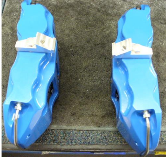
Hose adaptors installed to allow use of original hoses
