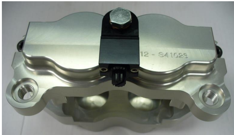
Caliper with CSV installed.
