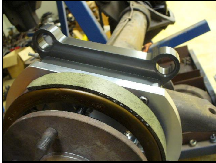
Park brake assembly correctly installed
