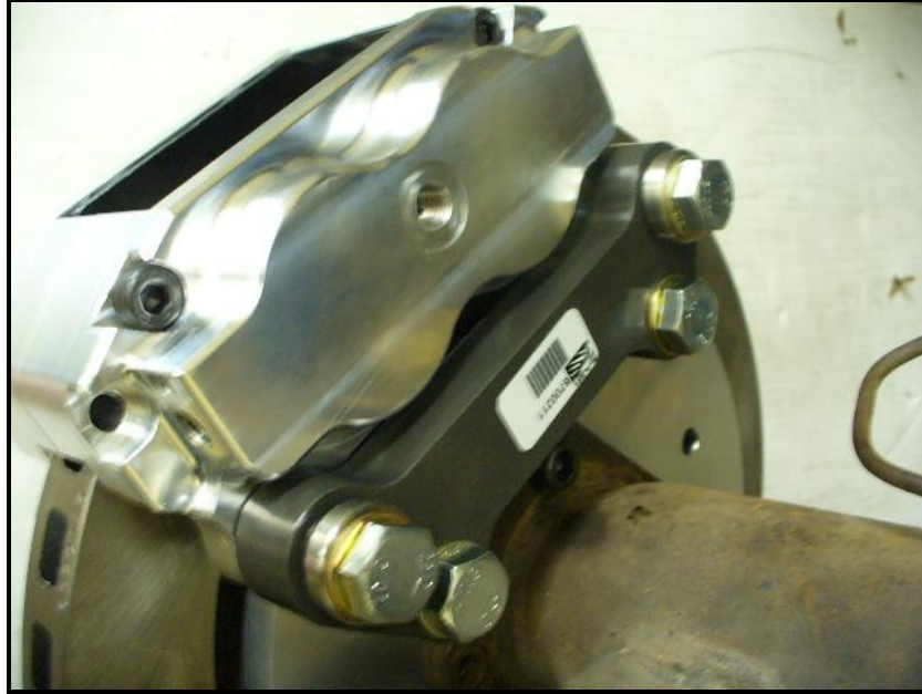
Caliper installed on intermediate bracket.
