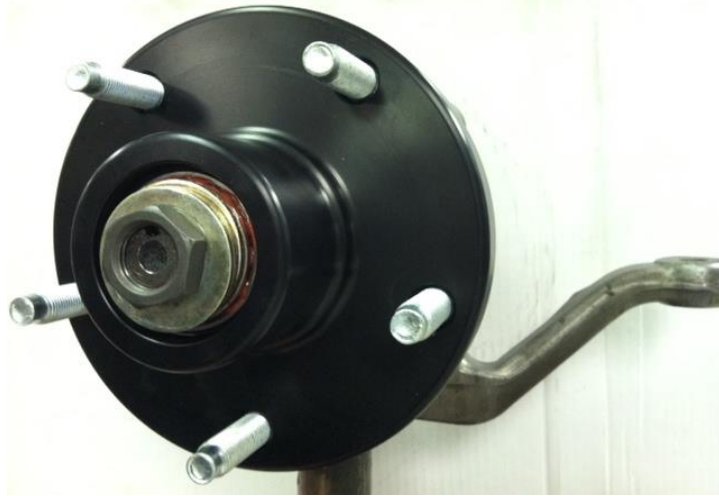
Hub installed, left or drivers side. Caliper mounts ahead of the centerline.
