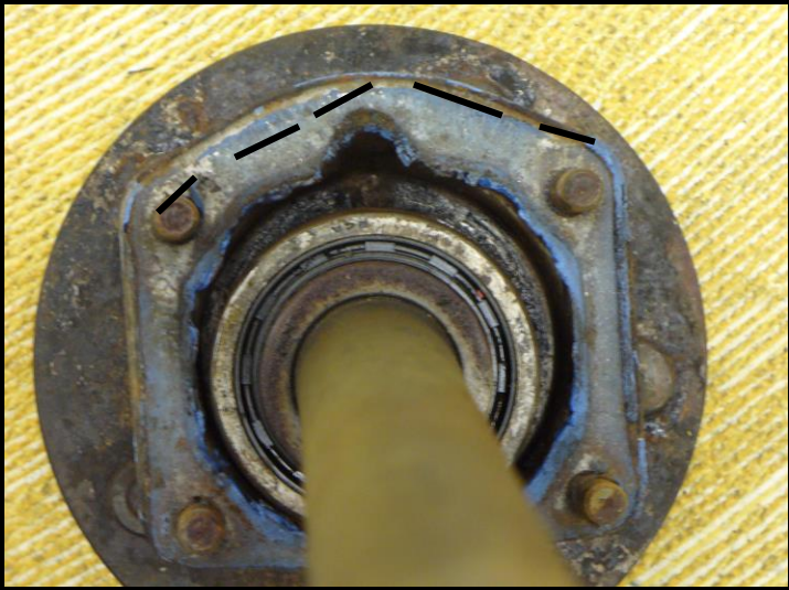
Trim along dashed line for fit (Your system may require similar trimming)
