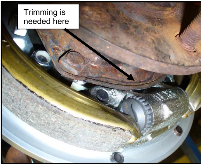
The steel plate is marked with a permanent marker for trimming
