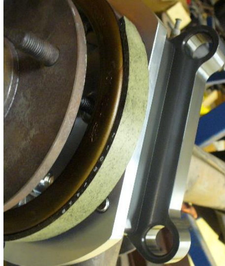
Park brake assembly correctly installed
