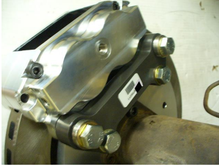
Caliper installed on intermediate bracket.
