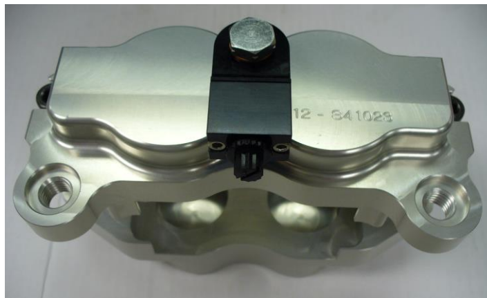
Caliper with CSV installed.
