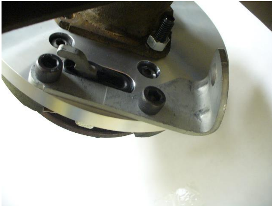
Park assembly installed on driver's side (Actuator is shown at the bottom)
