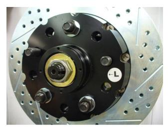
2. Install the caliper bracket using the supplied 7/16" VT (Vibra Tite, red thread coat) bolts, and washers. The top of the bracket will use the 7/16"- 20 X 1.0 bolt, and the bottom will use the 7/16"- 20 X 1.5 bolt. \*\*Note: The engraved part number on the bracket should face outboard, towards the hub. Torque bolts to 65 ft·lbs. See photo below for reference:
