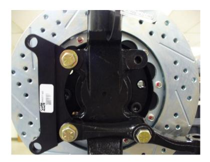
3. The caliper will now need to be installed using two 12mm X 25mm VT bolts with washers. Torque bolts to 83 ft·lbs. \*\*Note: All or most S4 Calipers are shipped with dual bleeders for orientation depending on the setup.
