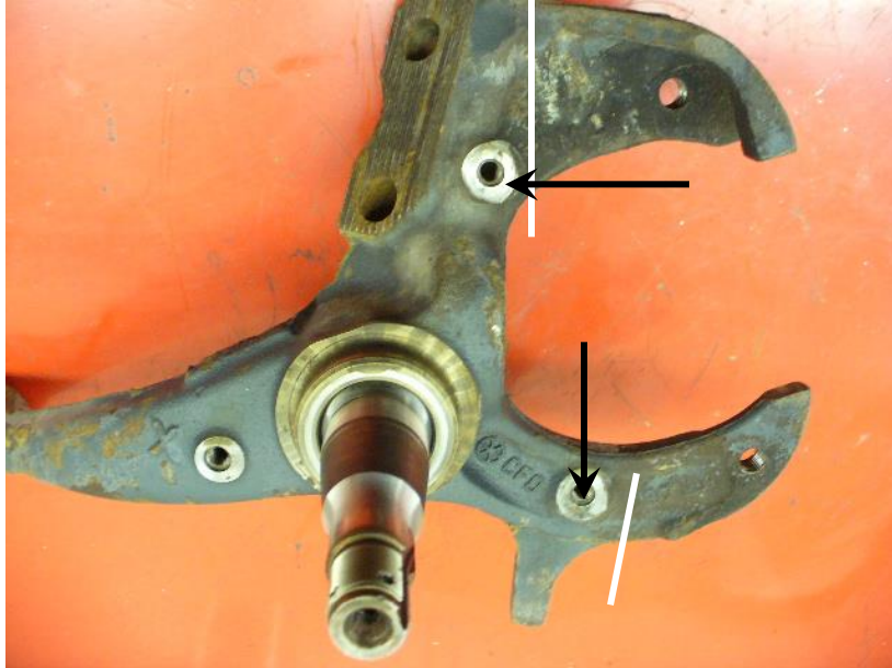
82-92 Camaro / Firebird Cut at white lines, drill and tap holes indicated by black arrows.
