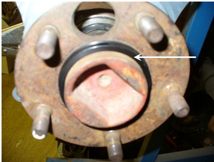
Black centering ring installed over rotor register.
