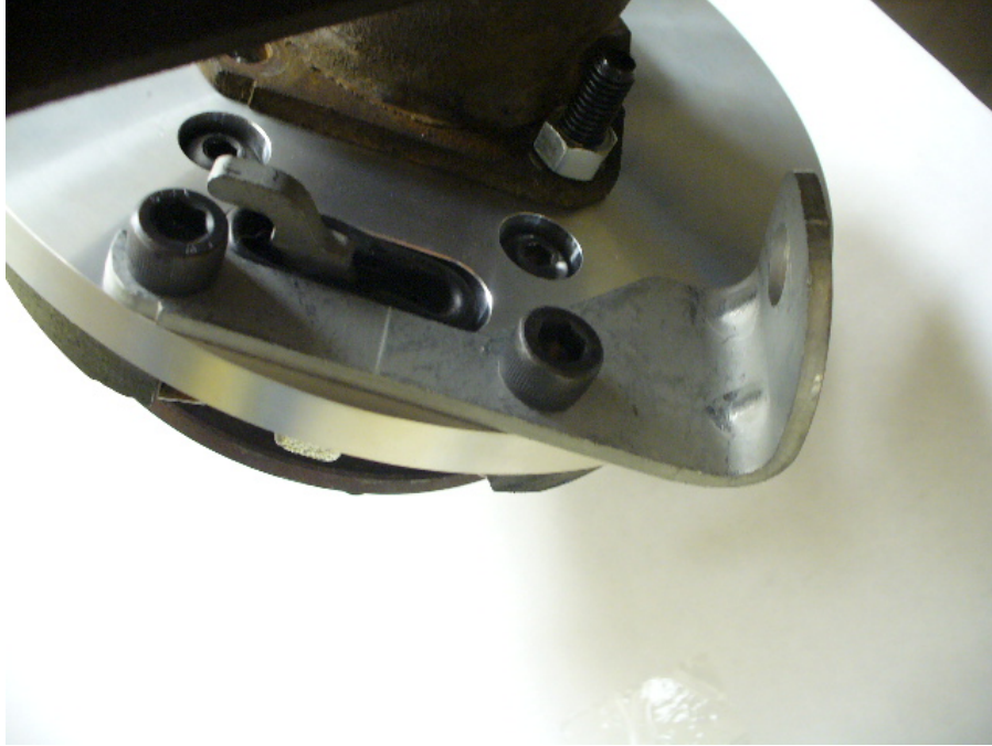
Park assembly installed on drivers side
