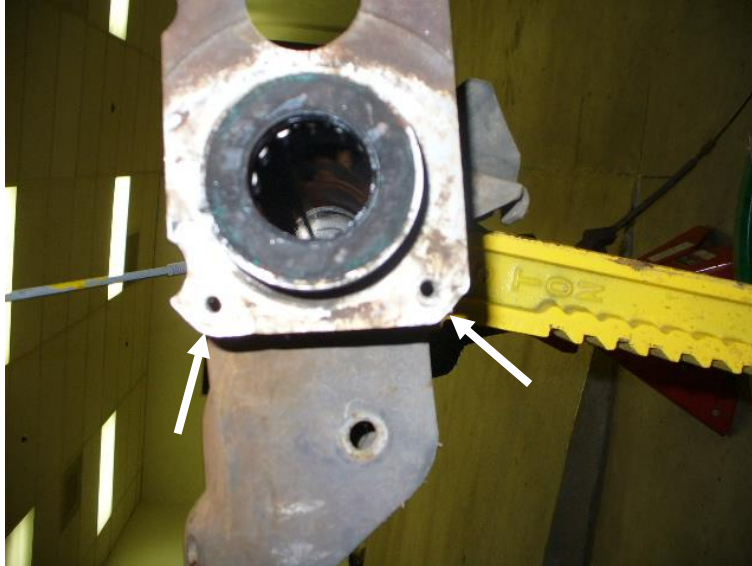
Figure 3: Drill these two holes to .375"
