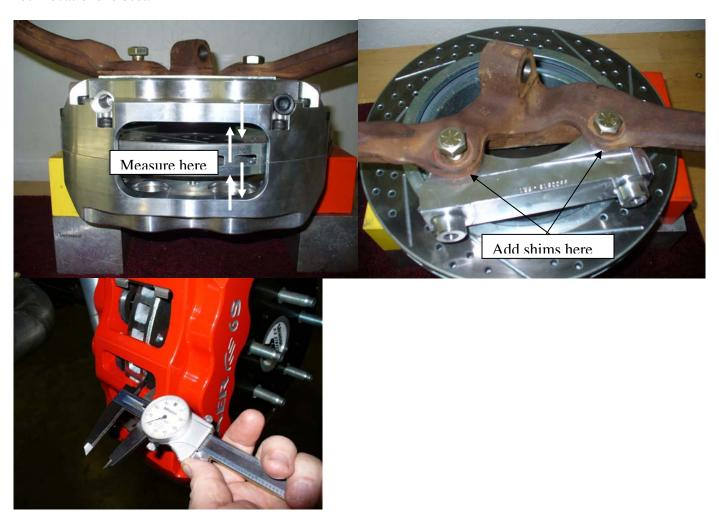
Once the proper fitment has been achieved torque the bracket bolts to 100ftlbs then tighten the caliper mount hardware to 85ftlbs.
