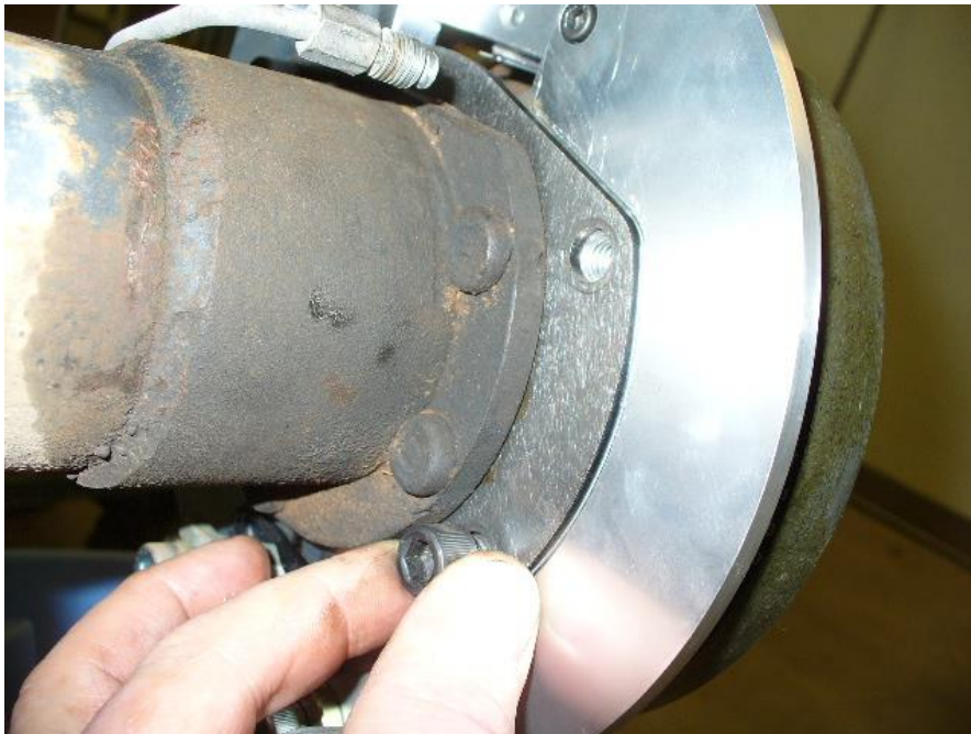
Remove allen head bolts that retain park brake assembly to intermediate plate.
